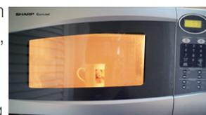
a. Bake the product for 10 min at 150°C (baking time and temperature must be adjusted according to the distance between the firing elements and your product).
